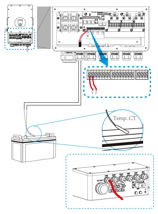
Without a remote temperature sensor, lead-acid batteries may undercharge or overcharge depending on the ambient temperature of the installation environment. This may result in a fire hazard.
