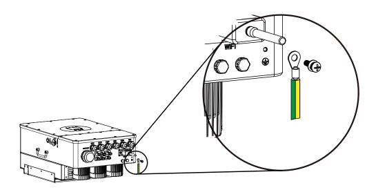
All neutrals can be linked together to maintain the neutral bond. When Neural Earth bond is required for 'Off-grid' operation, then it has to be removed on 'Grid-Tied' operation.
