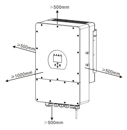
For proper heat dissipation, allow a clearance of approximately 500mm to the side, 500mm above and below the unit, and 1000mm to the front of the unit.
