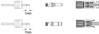
b) Crimp metal terminals with crimping pliers.
