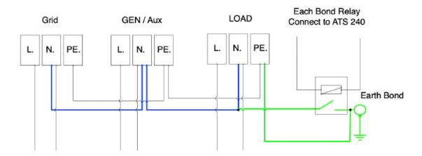
If an Earth Bond is required between neutral and earth and your system is a hybrid system then you can have a permanent earth wire since this can cause faults with an RCD before the inverter.
