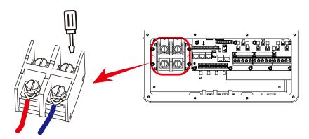
3) Make sure polarity is correct at both the battery and inverter terminals.
